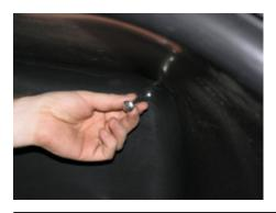
**Step 1.**Place S4 bolts in the four bottom holes inside the tub (2).
